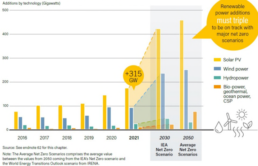
Annual Additions of Renewable Power Capacity, by Technology and Total, 2016-2021, and to Achieve Net Zero Scenarios for 2030 and 2050
